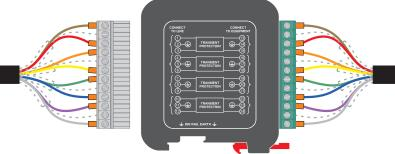
An ESP 06Q unit is capable of protecting: Four 2 wire systems
